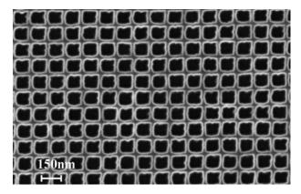
**Figure 3.** SEM image of square openings transferred into Pd hard mask by Ar ion milling.
