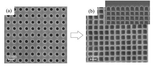
**Figure 1.** (a) A SEM image of  $\sim$ 75 nm openings on a square grid formed in PMMA using e-beam lithography. (b) Top view of 107 nm square openings on a 150 nm pitch after 12 min of self-limiting Ar<sup>+</sup> ion milling at a beam energy of 500 eV. The insert shows the edge of the pattern where the self-limiting process fails.
