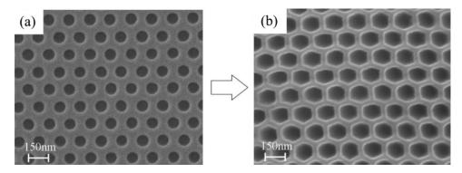
**Figure 2.** (a) An SEM image of  $\sim$ 85 nm openings (with  $\sigma$  = 2.0 nm) on a hexagonal grid formed in PMMA using e-beam lithography. (b) Top view of 105 nm (with  $\sigma$  = 3.0 nm) hexagonal openings on a 150 nm pitch after 12 min of self-limiting Ar<sup>+</sup> ion milling at a beam energy of 500 eV.
